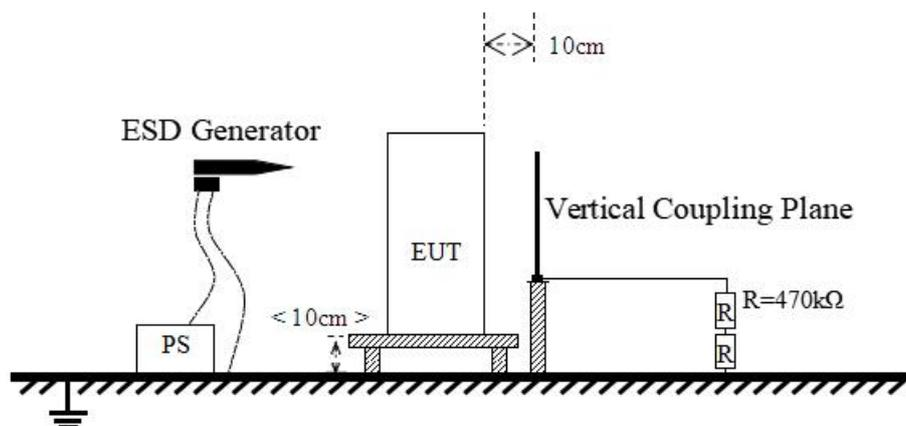
Test Setup 6 For Radiated Immunity Test
