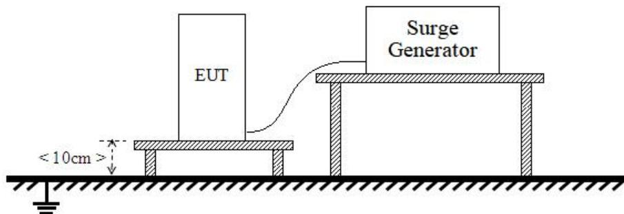
Test Setup 9 For Immunity to Conducted Disturbances Induced By RF Fields Test
