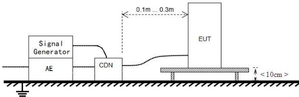
Test Setup 10 Power Frequency Magnetic Fields
