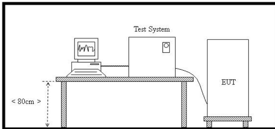
Test Setup 5 For Electrostatic Discharge Immunity Test
