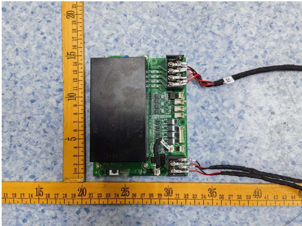
The back view of the mainboard (High Voltage Box)
