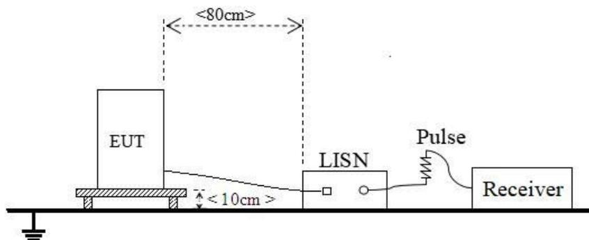
Test Setup 3 For Harmonic Current Emissions Measurement Test
