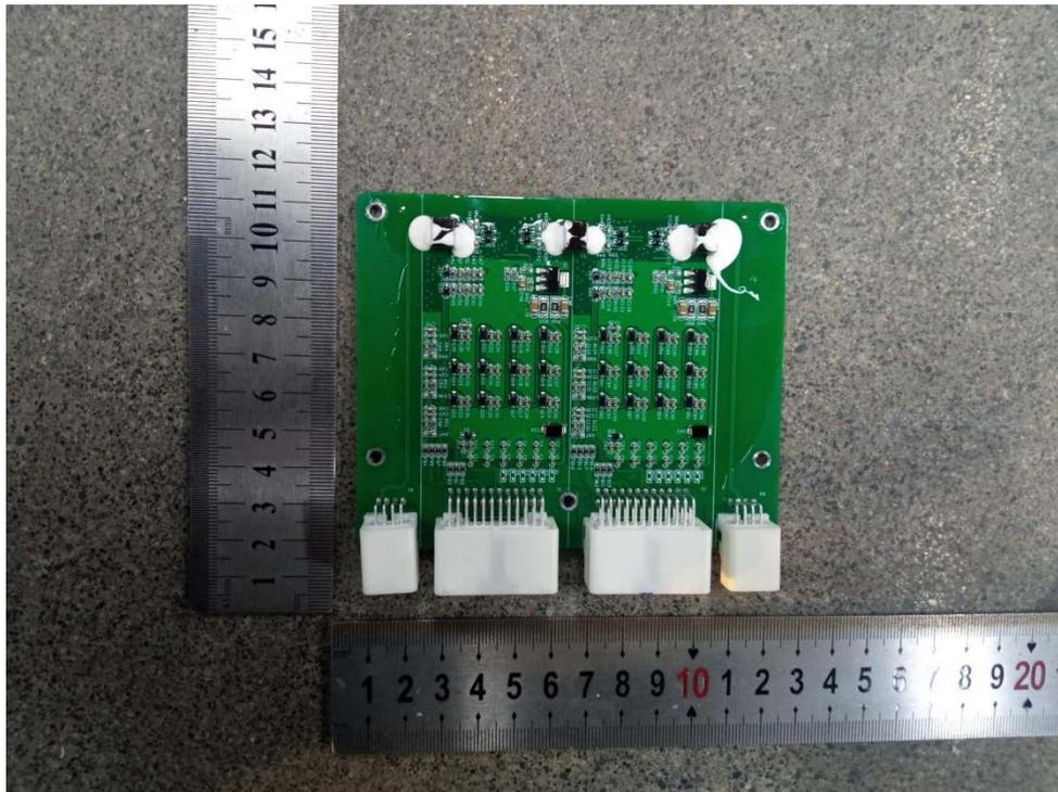
The back view of the mainboard (Battery Pack)
